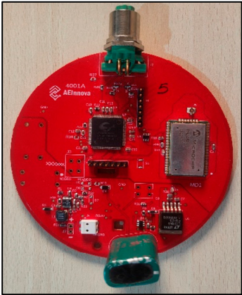
Figure 11. Main board soldered with all components ready for testing.
