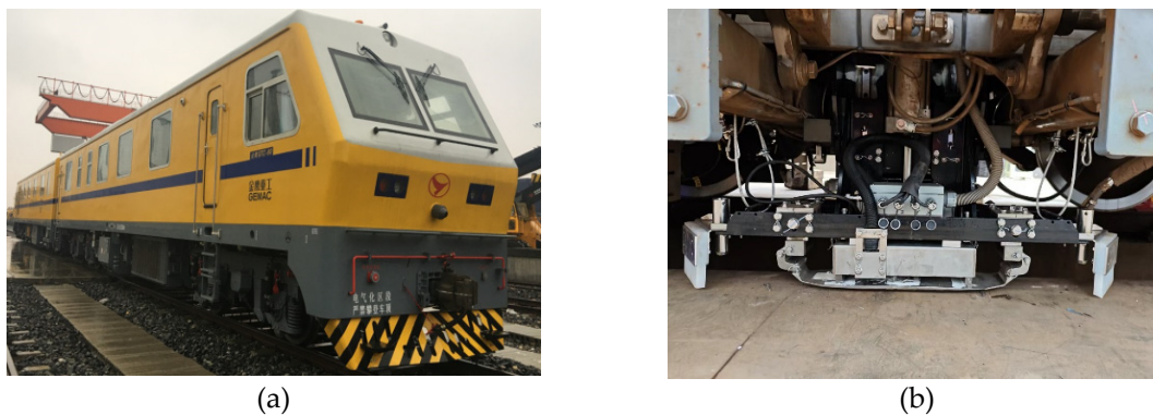
Figure 1. Rail magnetic flux leakage detection system: (a) GTC-80 rail inspection vehicle. (b) rail magnetic flux leakage (MFL) detection probe.
