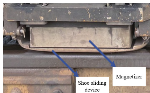
Figure 7. Physical image of core MFL detection probe in inspection vehicle.
