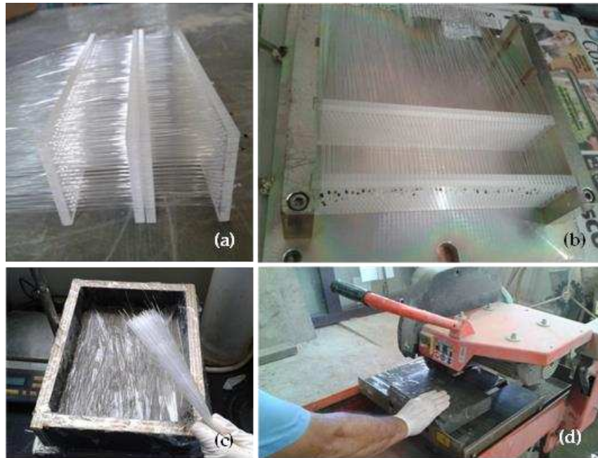
Figure 2. Molding process of translucent concretes: (a) and (b) using technology with sorted fibers; (c) and (d) adopting a method with random fibers [4,7].
