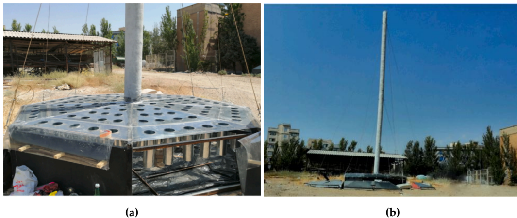
Figure 8. Insertion of hanging metallic tubes in the collector: (a) Side-view of hung metallic tubes from the canopy of the collector [79], (b) Overall view of the experimental solar chimney setup, reproduced with permission No. 5937201014767 [79]
