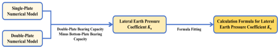
Figure 21. Derivation workflow for the lateral earth pressure coefficient formulation.
