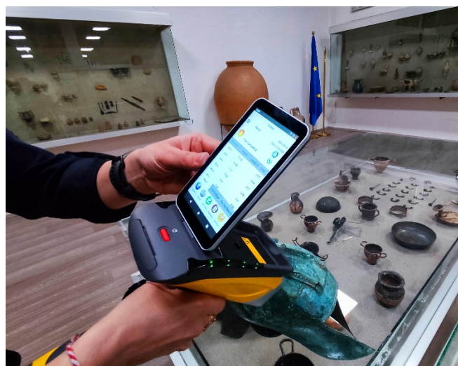
Figure 1. Explorer 5000 handheld XRF device (Skyray Instruments, Inc.) while conducting measurements at the Institute of Archaeology. (photo taken by the authors).
