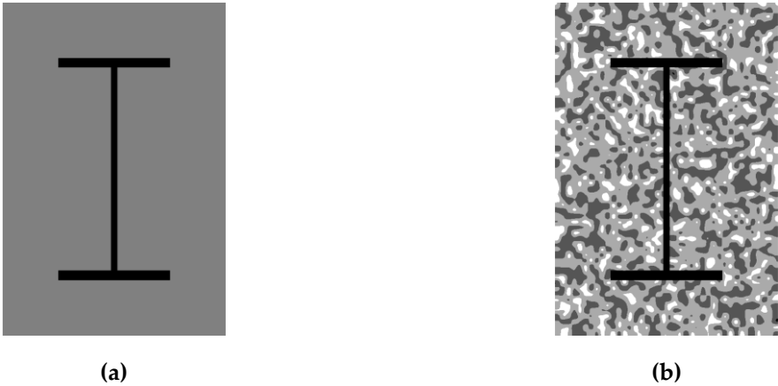
Figure 3. Spatial distribution of the shear modulus G(y,z) in the hybrid cross-section: (a) uniform matrix modulus G_m ; (b) heterogeneous matrix modulus G_m(y,z) derived from a density-dependent relation.
