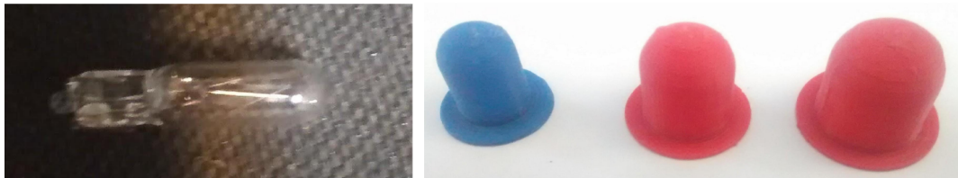
Figure 7. T5 car dashboard lamp 12V/12W (left); lamp caps: 8mm, 10mm, and 12mm, from left to right (right).
