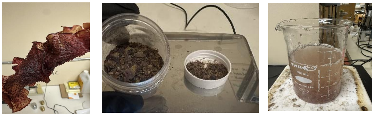
Figure 1. RA solution preparation method. This figure outlines the extraction steps used to obtain RA polysaccharides, including washing, drying, blending, heating, filtering, and centrifugation. The final drying and grinding stages produce the solid polymer material used in subsequent film fabrication.
