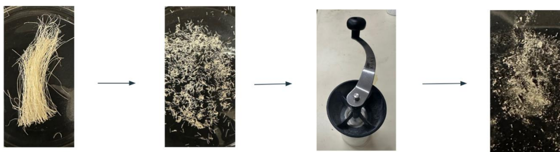
Figure 2. The sisal fiber preparation method involves cutting raw fibers into short segments and then grinding them to a fine powder using a ceramic burr grinder. This process improves the fiber dispersion within the RA–glycerol matrix.
