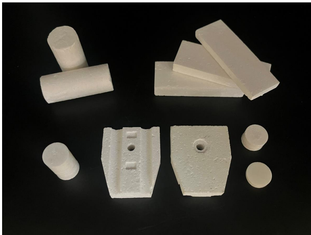
Figure 6. In the center, a high-temperature ceramic protection for a thermocouple fabricated using CAD/CAM. Surrounding it are various test specimens produced using pressing dies: cylindrical, plate-type, and disc-shaped specimens. All figures are made from recycled zirconia.
