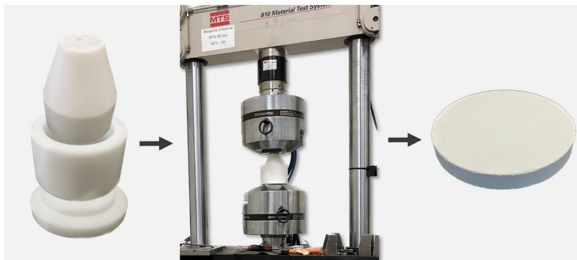
Figure 3. On the left, a custom-made Delrin plastic mold that shapes compressed powder into discs. In the middle, the mold containing the powder is placed under pressure in the press. On the right, a disc made from recycled zirconia powder is presented.
