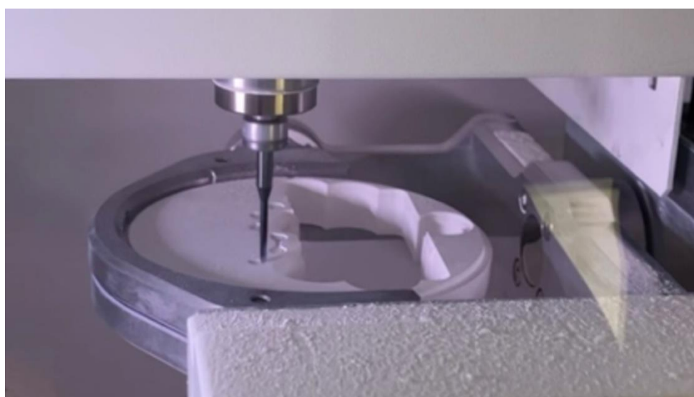
Figure 1. Standard milling process of a commercial 98 mm diameter zirconia disc in a dental milling machine.
