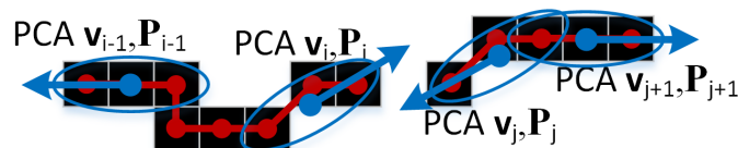
Figure 3. The end curve models are PCAs constructed from the first n^{pts} and last n^{pts} pixels of each curve (shown as blue ellipses) and aligned to point outwards from the curve.
