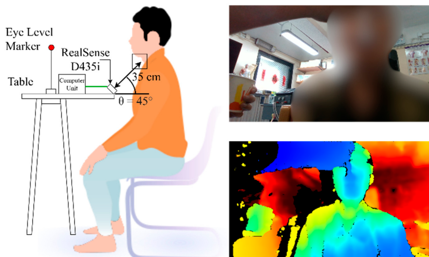
Figure 1. Experimental Setup for Data Collection. The participant was seated in a neutral position, with an RGB-D camera placed on a table approximately 35 cm from the target anatomical regions (lips, mandible, and throat) and angled at 45^\circ relative to the horizontal plane. The left side of the figure shows an illustrative screenshot displaying both the RGB and depth (D) channel outputs.
