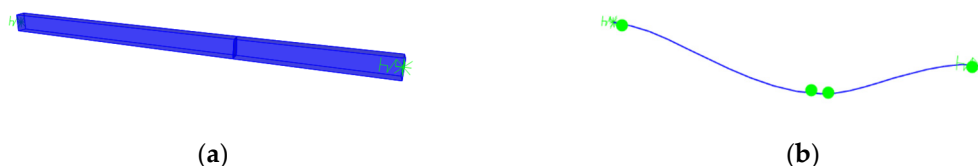
Figure 15. Double-span beam model: (a) Model layout; (b) Collapse mechanism and deformation mode.
