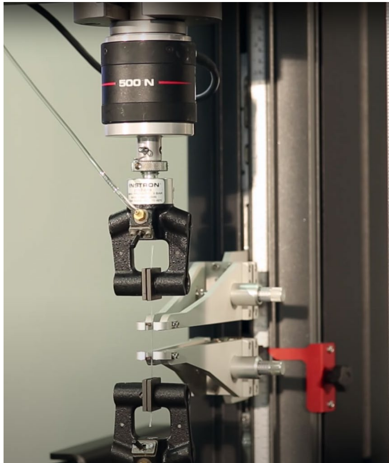
Figure 1. Destructive tensile testing of catheters.
