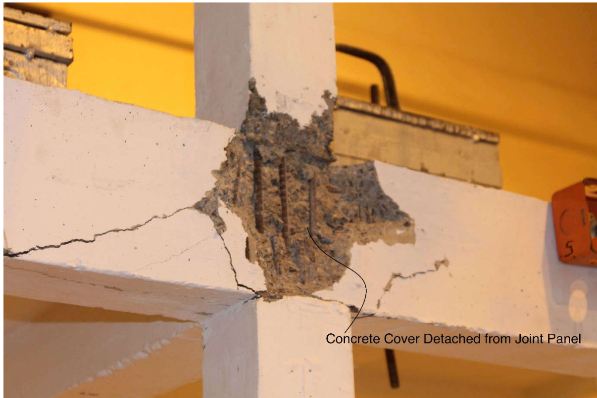
Figure 11. Extensive damage occurred at beam-column joint panel under test run 4 (ref. Table 3).
