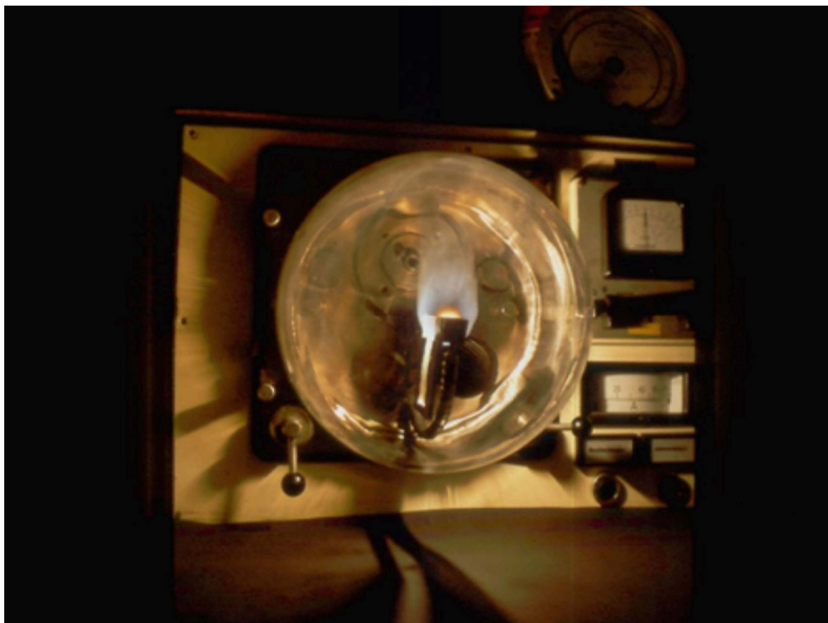
Figure 7. Fullerene generator "in action". It is a slightly modified carbon evaporator originally designed and used for TEM sample preparation. The device is currently showcased at the Deutsches Museum in Bonn, Germany..©Wolfgang Krätschmer[48].
