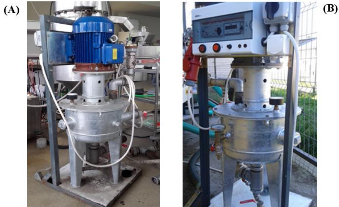
Figure 4. HC system used in research on an agricultural biogas plant in S2 (A – hydrodynamic cavitator, B – control and measurement module).
