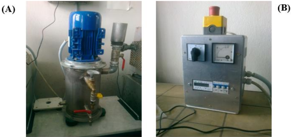
Figure 3. HC system used in laboratory tests conducted in S1. (A) hydrodynamic cavitator, (B) control and control and measurement module).
