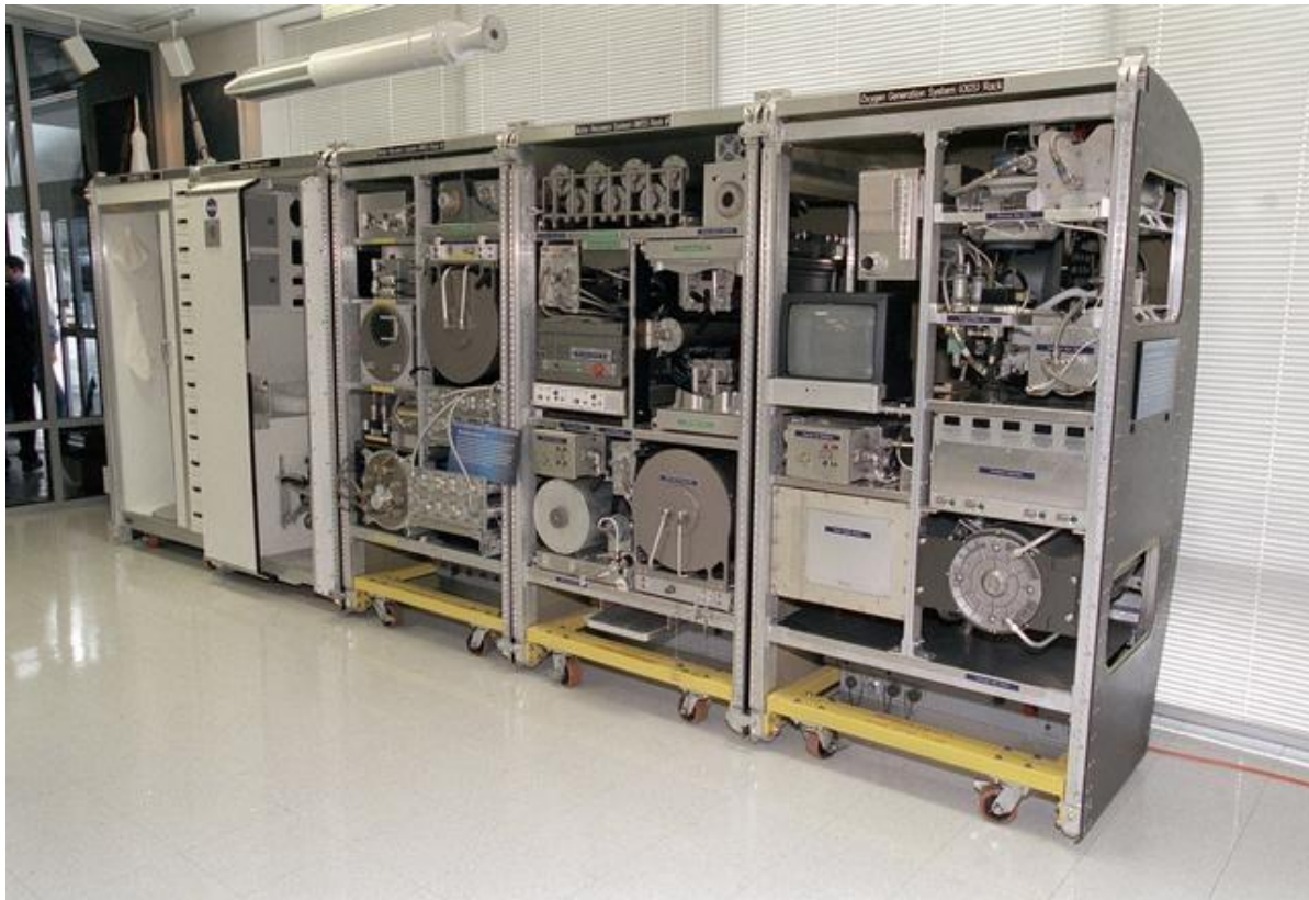
Figure 2. NASA Environmental Control and Life Support System (James E. Scarborough, Wikimedia Commons)- A working replica of ECLSS. The floor aligns five wheeled units, each resembling a double-door refrigerator. The leftmost unit, covered with a curtain, is the shower. Next is the waste management system with a closed white front panel. The two central units are water recovery systems, open at the front, revealing various metallic components. On the far right is the oxygen generation system, similar in design to the water recovery units.
