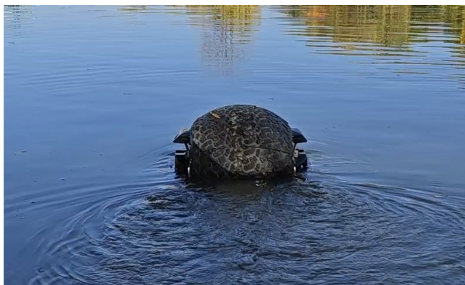
Figure 6. The amphibious spherical robot during water-based testing. (It is worth noting that the waterline appears to be slightly above the midpoint of the robot, indicating that more than half of the robot's body is submerged.)
