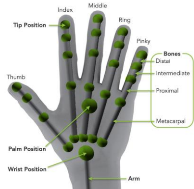
Figure 16. Leap Motion hand skeleton description (image source: https://www.ultraleap.com ).
