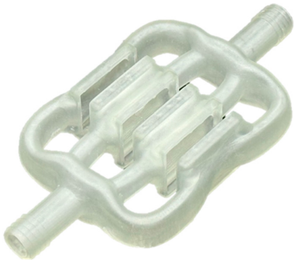
Figure 11. Fabricated prototype of the GD cooling manifold.
