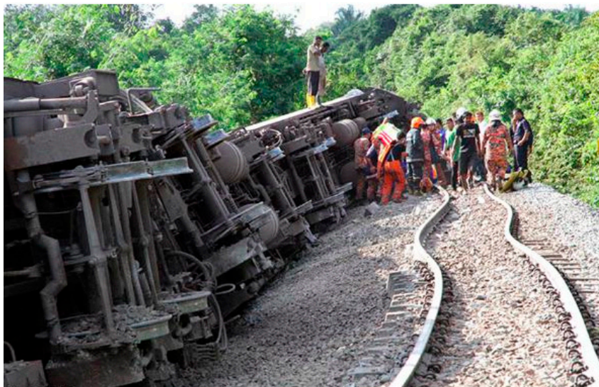
Figure 17. KTMB train derailed due to rail buckling and had landed on its side, trapping the driver and injuring about five passengers just before the Kempas, Johor station southern part of Malaysia (Courtesy: Malaysia Department of Public Works).
