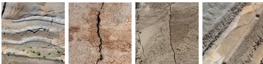
Figure 7. Examples of real-world open-pit mine surface crack images used for YOLOv11 performance evaluation.
