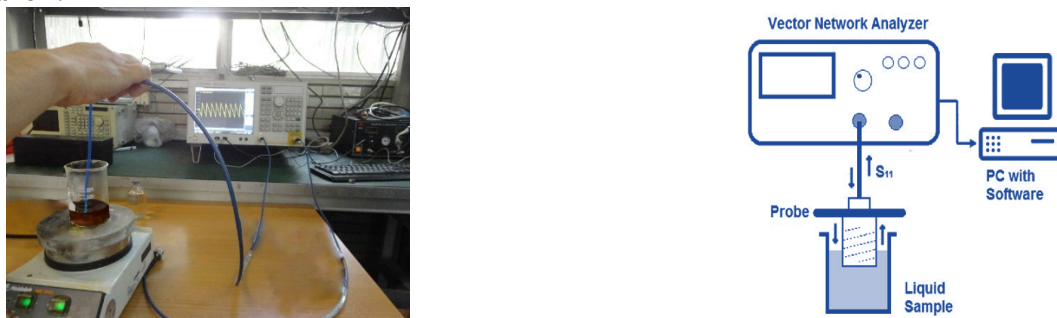
Figure 3. The experimental setup and its schematic view for measuring dielectric properties of lubricants.
