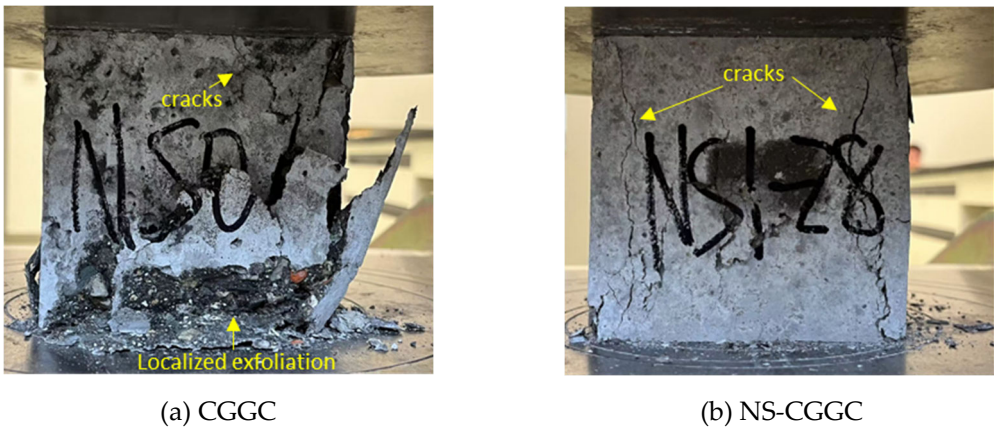
Figure 4 Morphology of compressive failure
