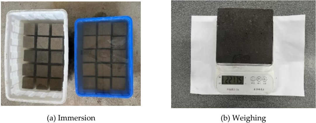
Figure 2. Sulfate erosion test
