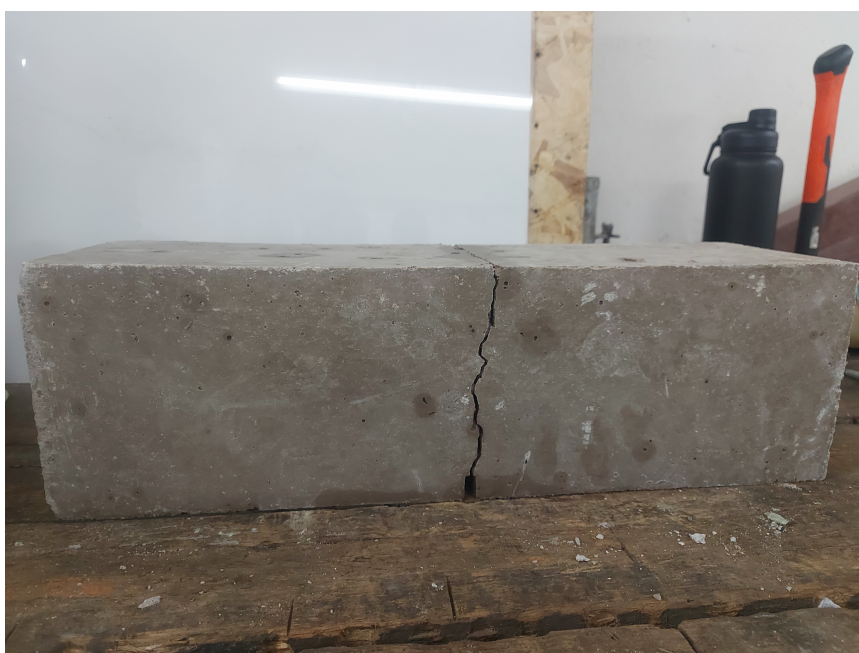
Figure 21. Crack of a plain concrete three-point single-edge-notched beam
