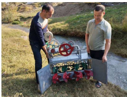
Figure 1. Micro hydroelectric power station based on a water engine.
