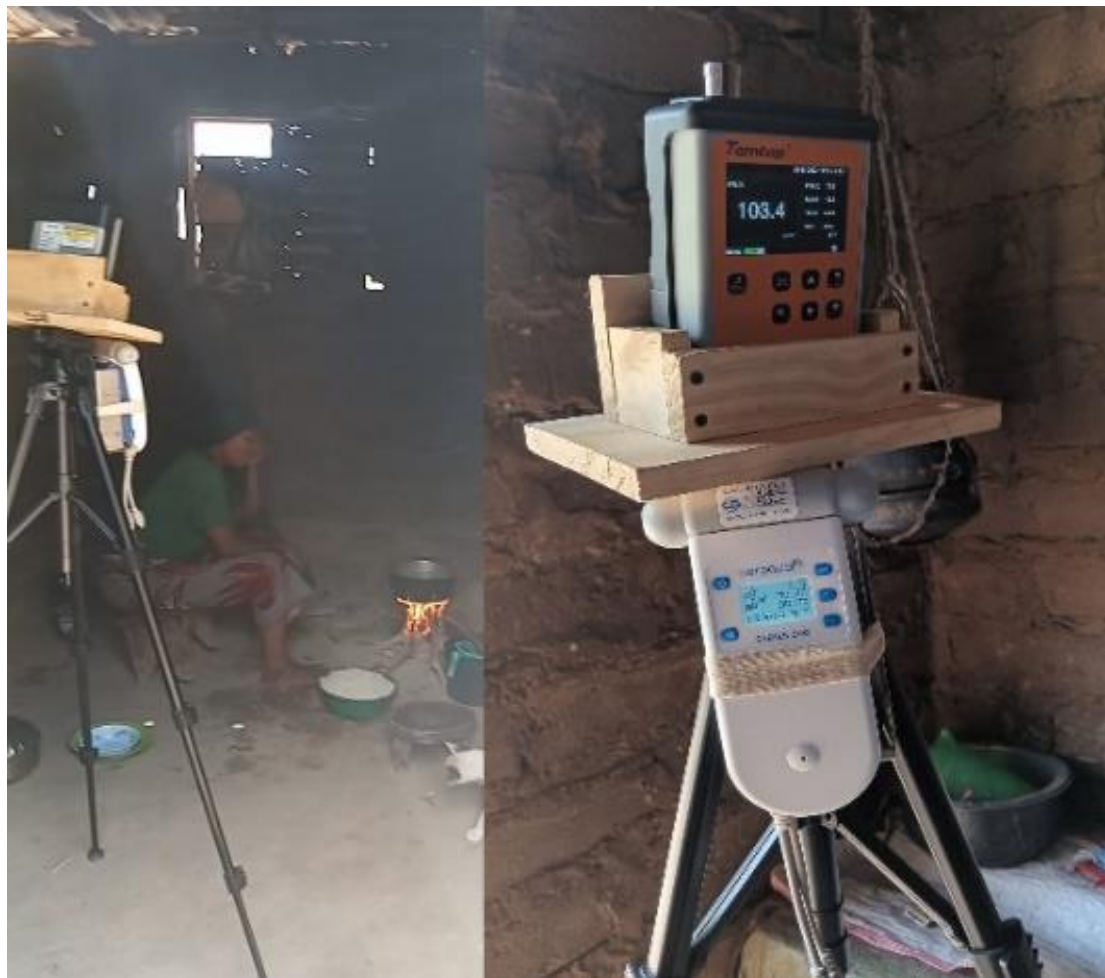
Figure 2. Positioning of air quality sampler.
