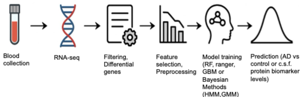
Figure 2. The stages of the transcriptomic biomarker discovery with machine learning. Created with Biorender.com.
