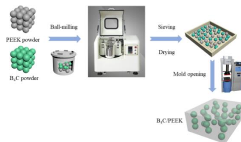
Figure 5. Preparation flow diagram of B 4 C/PEEK composite materials.
