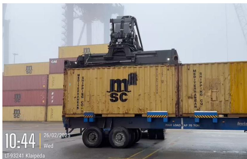
Figure 5. Rear impact between containers during loading onto a truck trailer platform.
