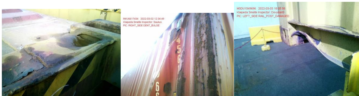
Figure 1. Examples of container damage resulting from bad handling operations.
