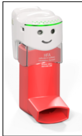
Figure 13. The CapMedic addon on a pMDI [83].
