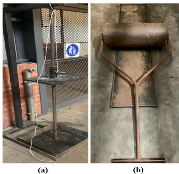
Figure 4. (a) Drop-weight impact rig used for conducting the drop shatter test. (b) Lawn roller and steel frame setup employed for compressive breakage experiments.
