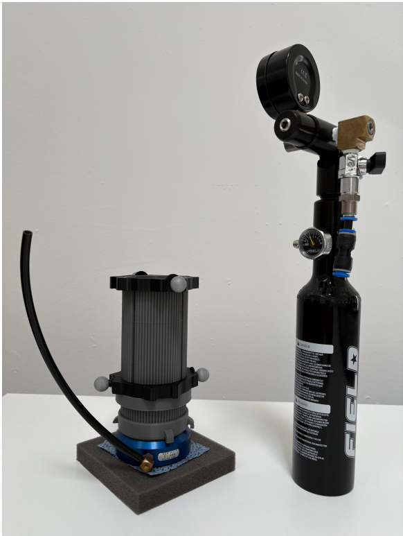
Figure 4. Air tank container with the air-bearing laid on a microfiber cloth, reflective markers (left) and pneumatic system (right).
