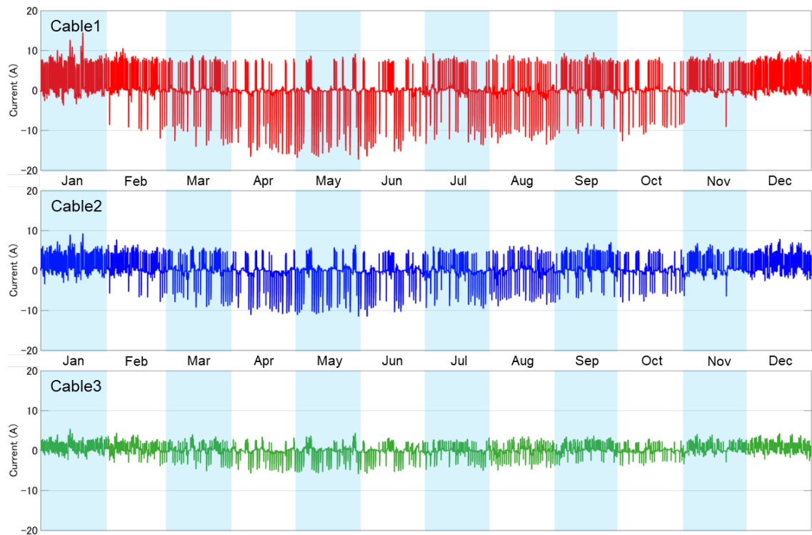
Figure 12. Current flowing through the baseline cables connecting the houses.
