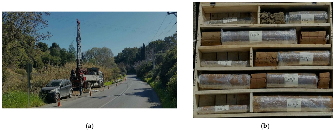
Figure 4. (a) Borehole drilling, (b) part of the borehole findings (Sand to Clayey geomaterial) is depicted [6].
