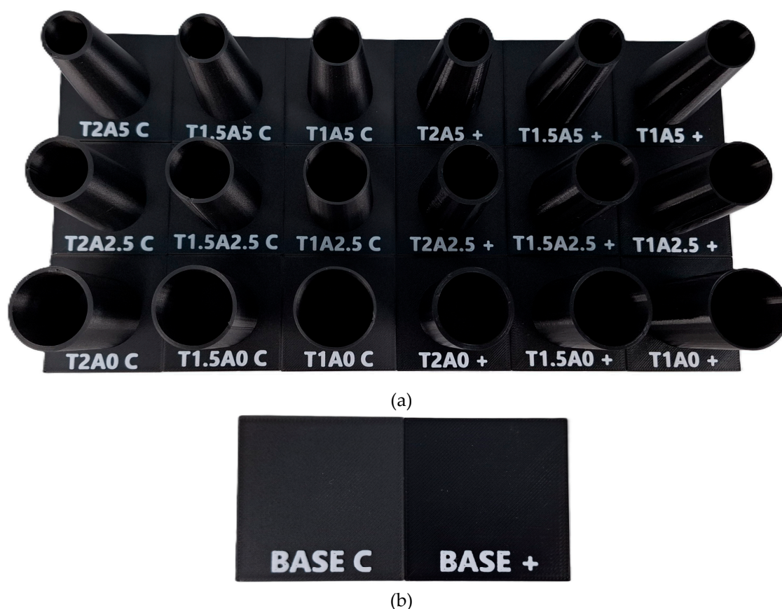
Figure 2. 3D printed (a) PLA+ and PLA-CF specimens; (b) PLA+ and PLA-CF bases.
