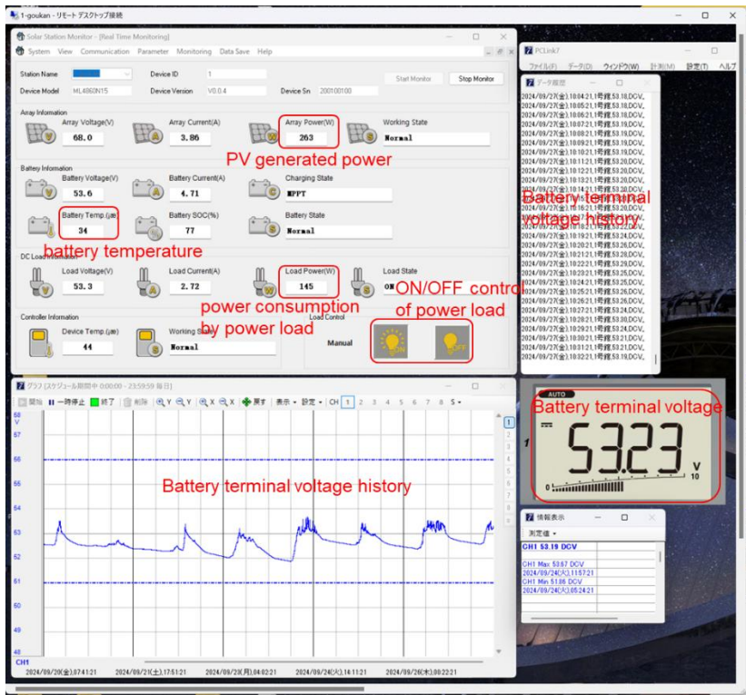
Figure 10. Monitor screen of the microgrid operation.
