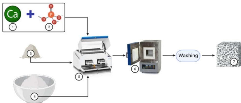
Figure 2. Schematic representation of the simplest algorithm of the dry method of hydroxyapatite production. 1 - source of calcium raw material (calcium hydroxide or calcium acetate monohydrate); 2 - source of phosphates (phosphorus pentoxide ammonium hydrophosphate); 3 - optional introduction of various salts, most often magnesium salts; 4 - pre-prepared calcium phosphate powders can also be used; 5 - intensive mechanical grinding (vibrating ball mill); 6 - high-temperature treatment of the powder mixture; 7 - transfer material in the form of primary raw material (adapted from [113]).
