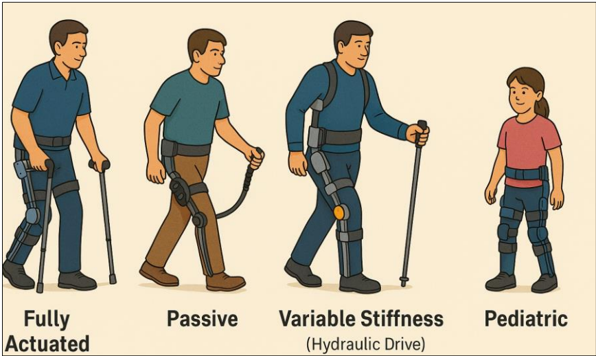
Figure 5. Hardware design and actuation strategies in lower limb exoskeletons. (1) Fully Actuated systems offering high control precision, (2) Passive designs utilizing mechanical elements like springs, (3) Variable Stiffness systems with hydraulic drives for adaptable force output, and (4) Pediatric-specific designs tailored for children, focusing on lightweight and ergonomic structure. The accompanying figure was created using tailored prompts in OpenAI’s ChatGPT environment [11].
