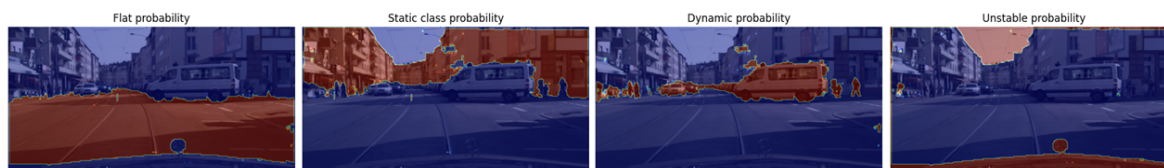
Figure 5. Visualization of the four semantic stability groups used for keypoint masking. From left to right: probability of flat regions (road, sidewalk), static structure (buildings, walls, poles), dynamic objects (cars, pedestrians, riders), and unstable or ambiguous regions (vegetation, sky, distant clutter). Red indicates high probability and blue low probability. These aggregated probabilities are thresholded to build the static/dynamic mask that filters out unstable keypoints before matching.
