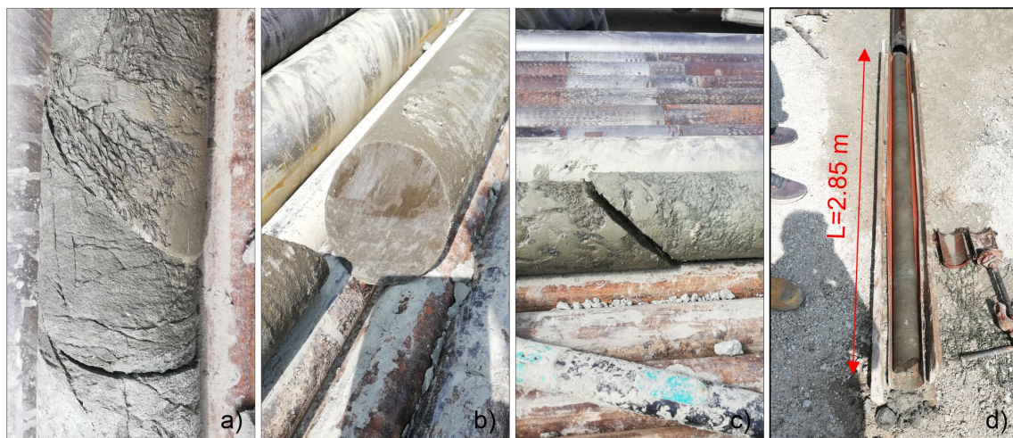
Figure 19. Details of the drilling of the bedrock. a), b) and c) Slickenside kinematic indicator. d) Extraction of an intact core in the S1 survey at -48.0 meters from ground level.
