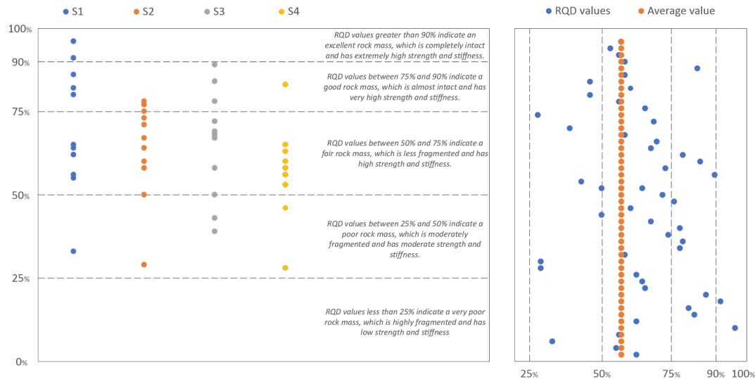
Figure 7. Distribution of RQD values calculated on each meter of core according to the single survey and representation of the average value.
