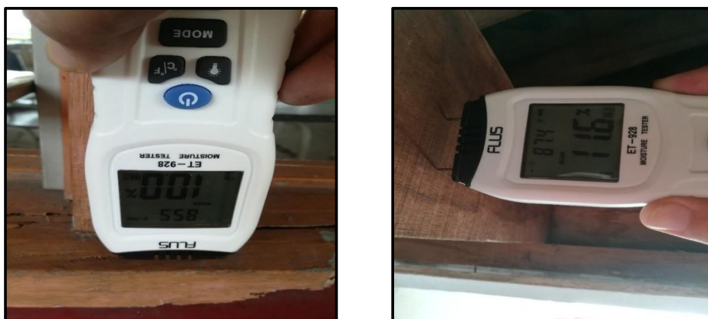
Figure 2. Various Assessment Moisture Contents Inspection.
