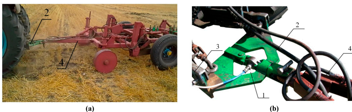
Figure 5. Components of the strain-gauge equipment installed on the tractor's hitch system. (a) General view; (b) Mutual arrangement of the strain-gauge equipment components, the tractor hitch system, and the field unit. 1 – Strain-gauge link; 2 – Plate for mounting the strain-gauge link; 3 – Tractor hitch system; 4 – Laboratory unit.
