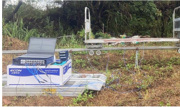
Figure 11. Trailer modal test site diagram.
