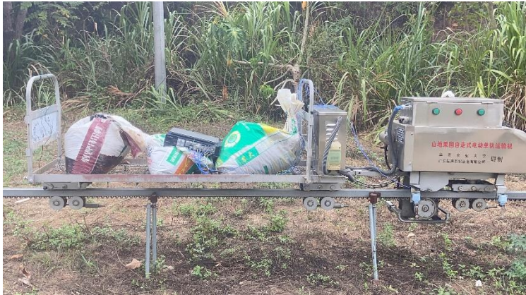
Figure 5. Vibration test site of transporter.
