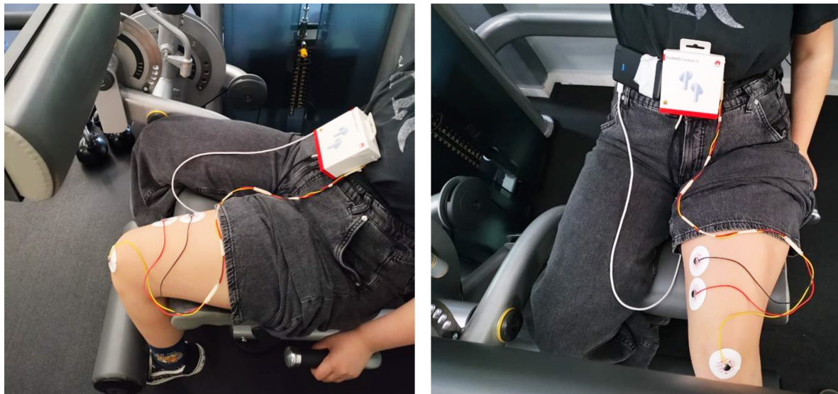
Figure 1. A participant preparing to perform the isometric leg-extension exercise. Experimental setup: our device inside a white box attached on the clothes of the subject, from which electrodes come out and are placed on surface of the muscle.
