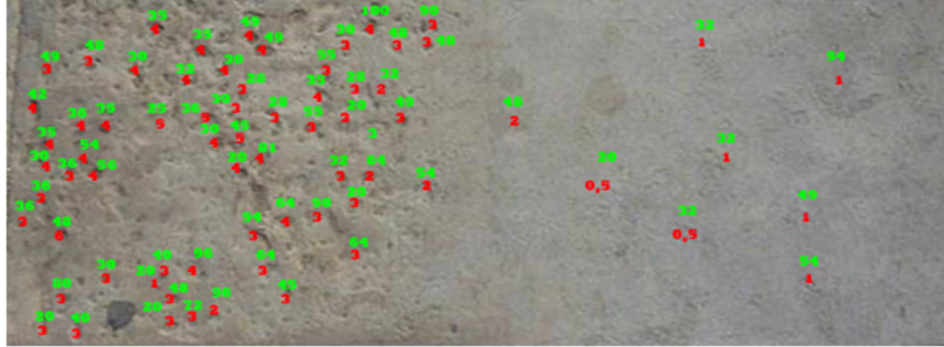
Figure 11. Calculation of erosion (volume of holes) in point 2: on the right, the part of the limestone pavement exposed to erosive agents for approximately 675 years; on the left, the part exposed since the time of construction.
