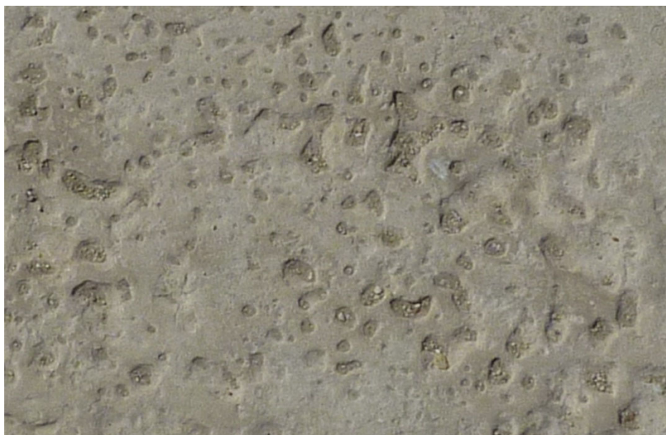
Figure 3. Pitting erosion on limestone rock.
