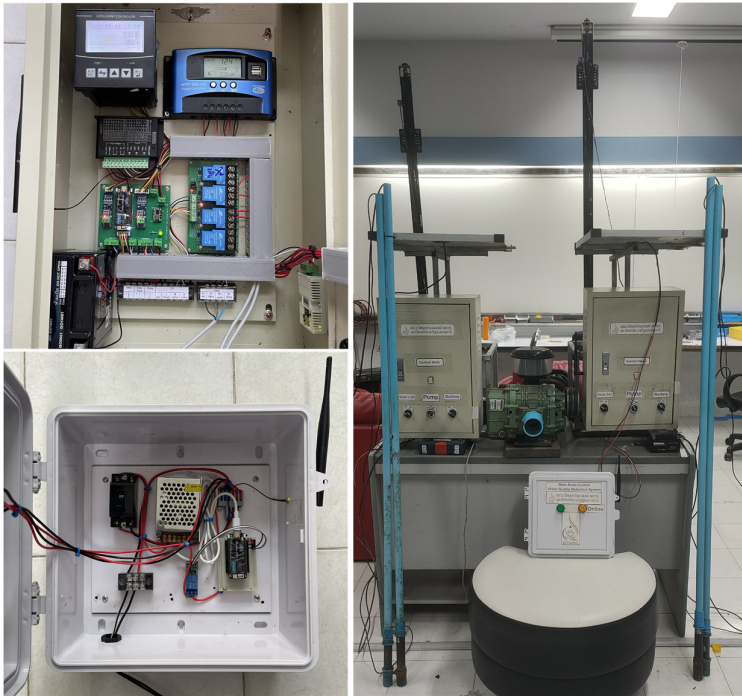
Figure 8. Prototype and electronic circuit connections of the main node and control node cabinet.
