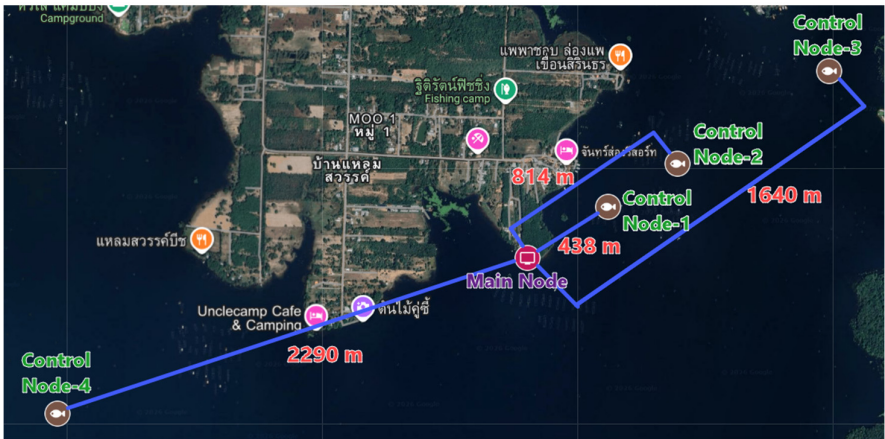
Figure 15. The coordinate location of the transmitting device, with the relative distances to the control node also provided.
