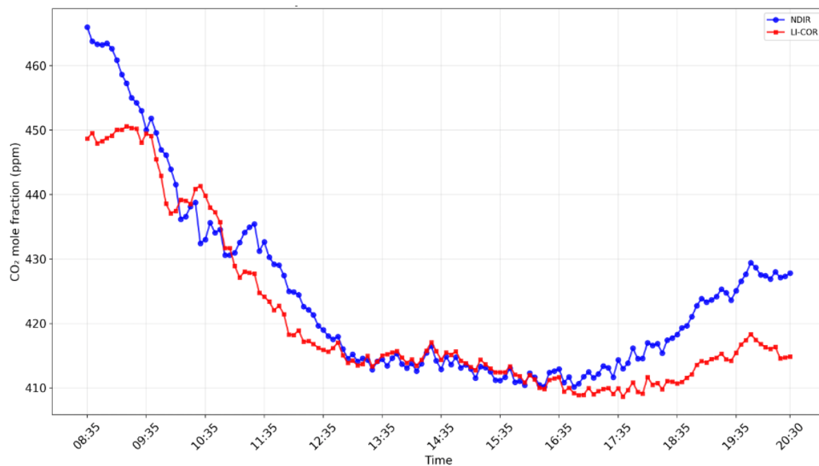
Figure 7. CO_2 mole fraction dynamics measured by LI-COR LI-7500A (red line) and NDIR (blue line) devices.
