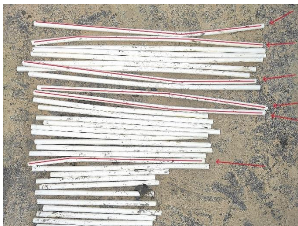
Figure 10. The bending state of the PVC pipe simulating the LDLP at the end of the test.
